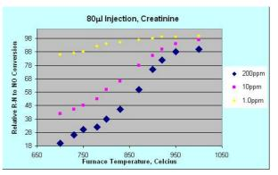
For most applications the TC catalytic furnace can be modified to allow it to perform both the TC and TN decompositions. However for higher level TN applications – up to 200mg/l – or highly particulated samples, a specialised TN oven is added.
