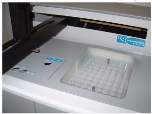
The Thermalox instruments utilize our Model 8000 XYZ autosampler. This gives maximum flexibility and allows a high degree of automation. Calibrants can be made up automatically; sparging, dilutions and sample agitation can easily be carried out.
