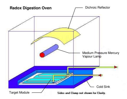
The Radox may be configured for continuous or batched digestion of aqueous matrix samples.
