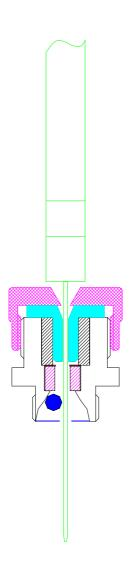
Replaces a conventional rubber septum to provide a long-life, bleedless alternative – without septum coring
