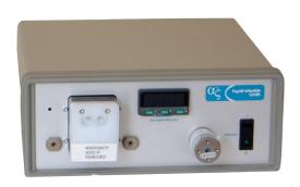
Developed initially to perform the hydrolysis of poly and meta-phosphate to orthophosphate, the 7601 Hydrolyser has a range of uses where the requirement is to "pressure-cook" a sample to speed up or create the conditions for a chemical reaction
