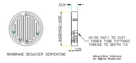
The case is manufactured from Stainless steel, with a permeable membrane fitted to a labyrinth. Liquid samples can be swiftly degassed – often without a separate vacuum source. All wetted parts are Teflon® and PEEK® with Viton® seals
